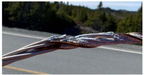
Figure 2: 2/0 ACSR Conductor Deterioration
