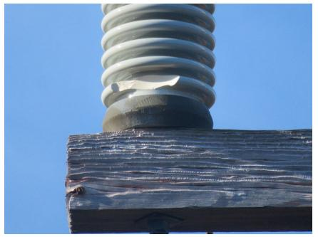
Figure B-3: Cracked Porcelain Insulator
