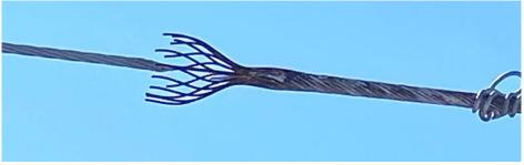
Figure 3: 2/0 ACSR Conductor Deterioration
