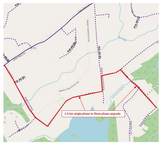
Figure 6 illustrates the work that would be required under this alternative.
