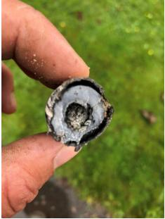
Figure 3: Loop 34 Primary Conductor Failure
