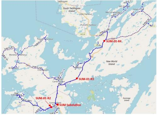
Figure 1 is a map illustrating the route of distribution feeder SUM-01 and its service area.<sup>8</sup>
